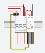
VI. Connect the voltage connection. Ensure polarities are correct
